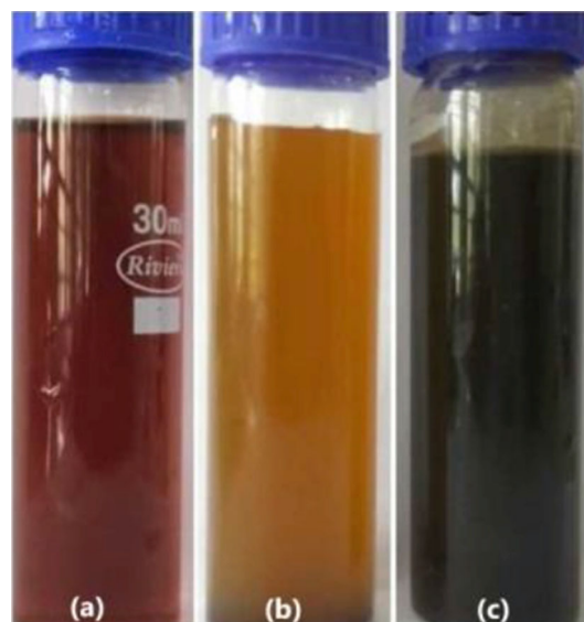
Figure 1. (a) Tea leaf solution, (b) GO solution and (c) rGO solution.
